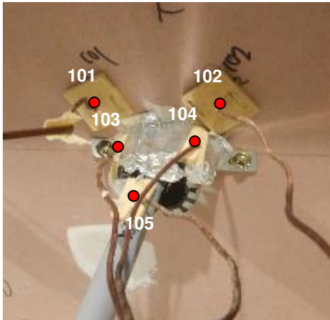
Figure 9 Penetration system F
