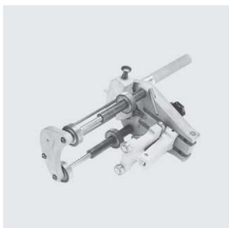
For the reliable removal of the oxide layer on spigot fittings. Additionally it is also possible to scrape HDPE and PE-Xa-pipes (maximum along half length of couplers d 710). Scraper blade made of carbide for a long life. Even swarf removal thanks to a spring-loaded scraper blade and automatic feed. Includes a replacement blade. The tool is delivered in a transport box.
