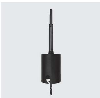
Drilling equipment FWAB for drilling HDPE pipes in unpressurised condition through the outlet spigot of FRIALEN XL spigot saddles SA XL, FRIALEN spigot saddles SA UNI as well as FRIAFIT sewage saddles ASA VL. Drive with drilling machine. Consisting of hole saw (nominal width-related), hole saw adapter SDS max, extension for hole saw adapter, centre drill with ejector and retaining shell, and 1 x hexagon wrench. The tool is delivered in a transport box.
