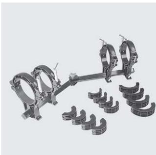
Alignment clamp with angle adjustment (45°/90°) and two clamping elements for heating coil fusion couplers, reducers, and 45° and 90° elbows d 63, d 90, d 125, and d 180. Reduction shells can be inserted for various sizes. Delivered in a practical carrier bag.
