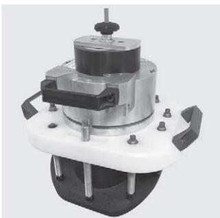
Clamping unit designed for FRIAFIT sewage saddles ASA TL and FRIAFIT transition saddles ASA TL/KG, specifically for HDPE Close Fit Inliners DN 200 to DN 500 and for HDPE pipes d 630. For clamping and creating the necessary joining pressure during fusion. Comprising ASATOP clamping unit with toggle anchor, hole saw ( $\varnothing$  95 mm) with hole saw adapter SDS, centre drill and extension, and compressed air pump. The tool is delivered in a transport box.
