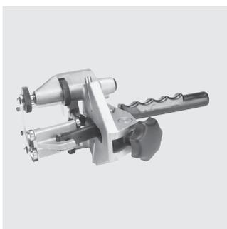
For the reliable removal of the oxide layer of HDPE and PE-Xa pipes. Scraper blade made of carbide for a long life. Even swarf removal thanks to a spring-loaded scraper blade and automatic feed. Includes a replacement blade. The tool is delivered in a transport box.
