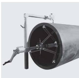
For the reliable removal of the oxide layer of large pipes made of HDPE in the diameter range d 800 to d 1200, SDR11-SDR33. Modular design for easy handling and quick assembly. Diameter adjustment through quick setting. Center-supported drive via hand crank. Automatic compensation of pipe out-of-roundness and tolerances through spring-supported adjustable blade unit. Scraper blade designed as turning blade with 2 cutting edges (twice the service life). The tool is delivered in a transport box.
