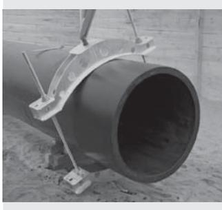
For the retrospective rounding of HDPE pipes. These rounding clamps are also available for hire.
