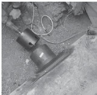
**PE 100****Maximum working pressure 2,5 bar (sewage)**
