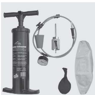
Repair kit for containing residual water during repair and installation work on d 90 - d 900 HDPE water pipes. Consisting of a universal repair set with pump, pressure gauge, drill, connecting hose, and additionally repair balloons for each pipe dimensions. Optional extension set for the connection of an additional repair balloon, consisting of additional connection hose of 3m and pressure gauge.
