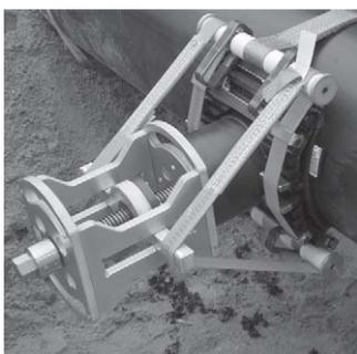
For the assembly of FRIALEN spigot saddles SA UNI d 250 – d 900 with outlet d 90, d 110, d 125 and d 160. The tool is delivered in a transport box.
