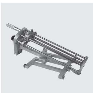
For the reliable removal of the oxide layer of HDPE pipes for half or entire coupler length. Scraper blade made of carbide for a long life. Even swarf removal thanks to a spring-loaded scraper blade and automatic feed. Includes a replacement blade. The tool is delivered in a transport box.
