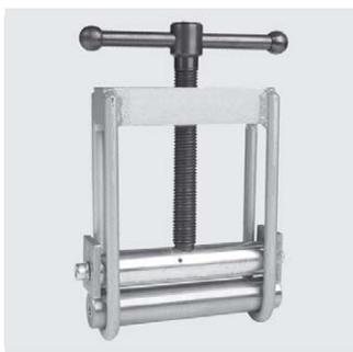
Manual squeeze-off tool for the temporary shutoff of HDPE and PE-Xa pipes d 63–d 125 in SDR 11 and SDR 17.6.
