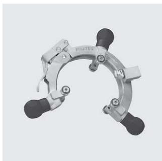
Dimension-bound scraper tool for the reliable removal of the oxide layer of HDPE and PE-Xa pipe ends and in the saddle area. Scraper blade designed as turning blade with 2 blades (twice the service life). Easy clamping thanks to the open design of the scraper tool. The tool is delivered in a transport box.
