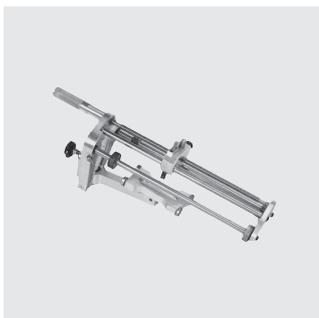
For the reliable removal of the oxide layer of HDPE and PE-Xa pipes for half or entire coupler length. Scraper blade made of carbide for a long life. Even swarf removal thanks to a spring-loaded scraper blade and automatic feed. Includes a replacement blade. The tool is delivered in a transport box.
