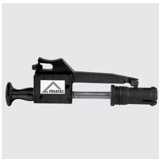
Dimension-bound compact scraper tool for the reliable removal of the oxide layer of HDPE and PE-Xa pipes and at the outlets of FRIALEN safety fittings. Super long scraping length, in the diameter d 32 also for FRIALONG long couplers. Scraper blade made of carbide with 2 edges (twice the service life). Automatic compensation of pipe out-of-roundness and tolerances. Manual operation, with hand crank or cordless screwdriver.
