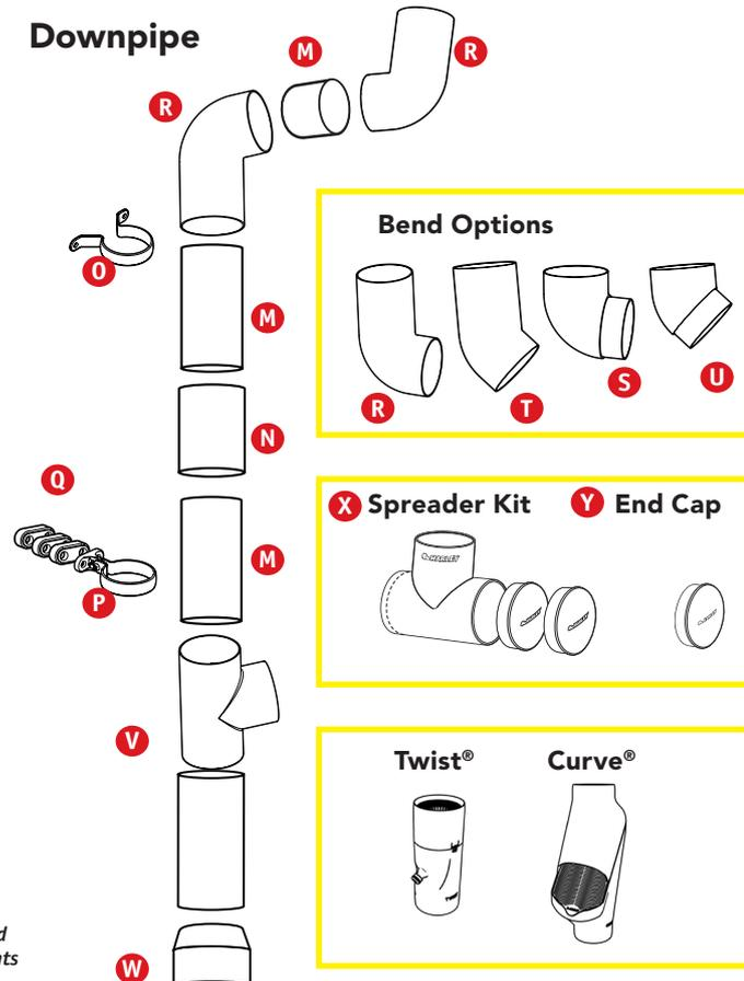
NOTE: Marley's Typhoon® spouting system and RP80® 80mm round downpipe systems have been used as examples in the diagrams shown on this page - shape, functionality and availability of components will vary depending on the specific spouting or downpipe system.
