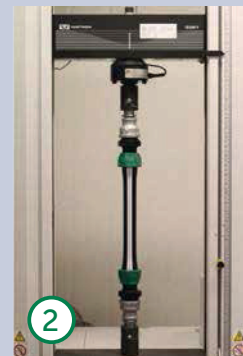
2 Pipe and fitting under high load (see massive elongation of pipe)
