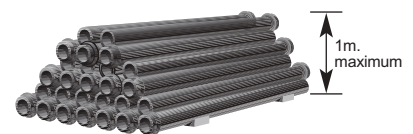
Individual pipe stacks on site
