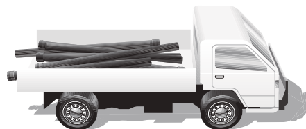
Incorrect way to load pipes
