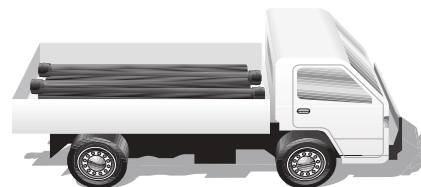
Correct way to load pipes
