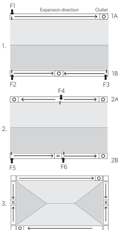
1A. For an expansion outlet positioned at one end of a spouting run, the expansion will be directed from the stopend to the expansion outlet. Fix at location **F1**.
