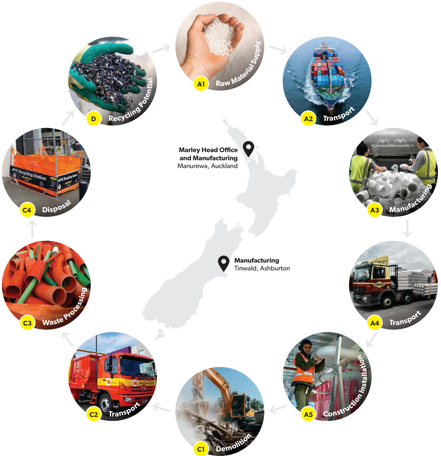
Figure 3. Marley PVC pipe manufacturing sites and showing modules related to the EPD
