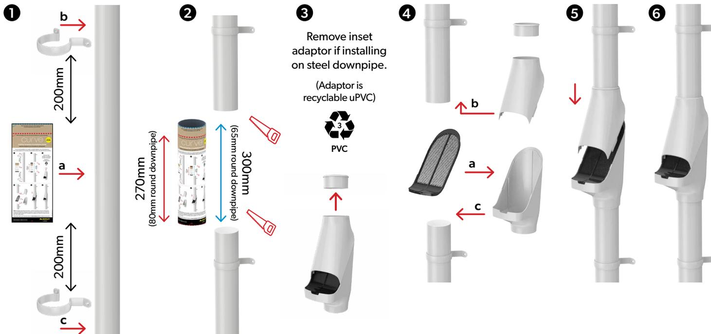
**Metal Downpipes:** Curve is now available to be fitted to 80mm metal downpipe systems by removing the top inset adaptor, (3).
